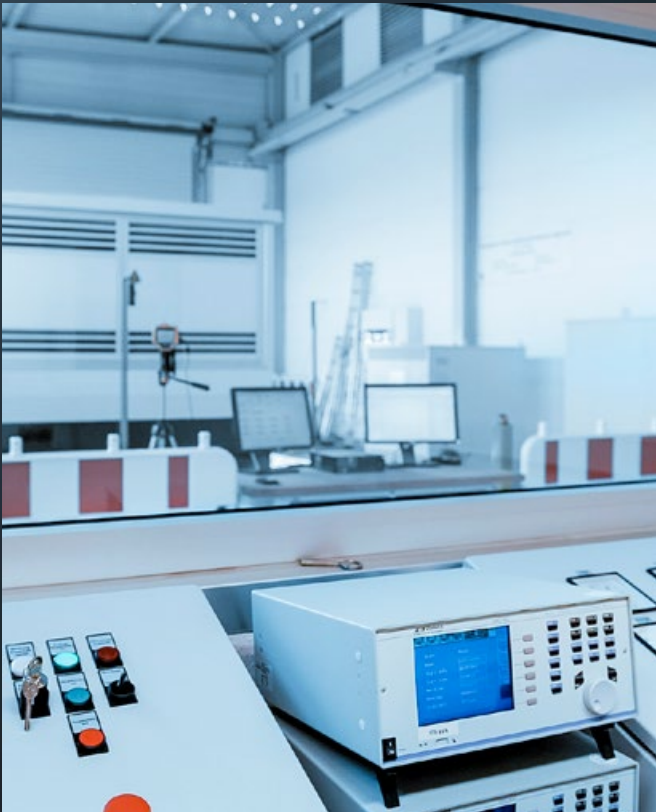
Test arrangement for temperature rise Test
