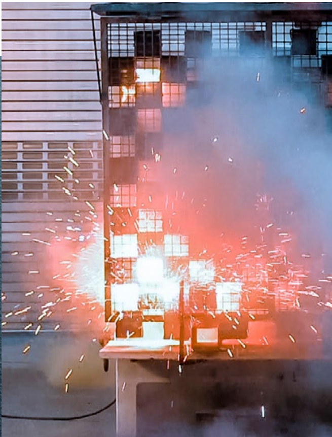
Internal arc test arrangement IAC-A 20 kA/1s, according to IEC 62271-202.
