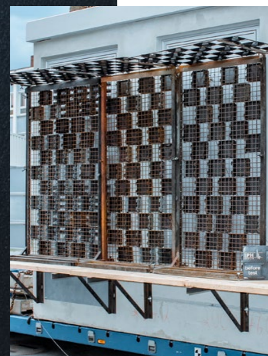
Internal arc test arrangement IAC-B 20 kA/1s, according to IEC 62271-202.
