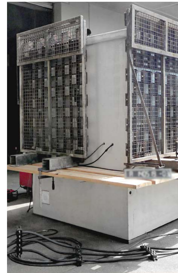
Fault arc test of a walk-in station with IAC-B 20 kA 1s (pedestrian protection)
