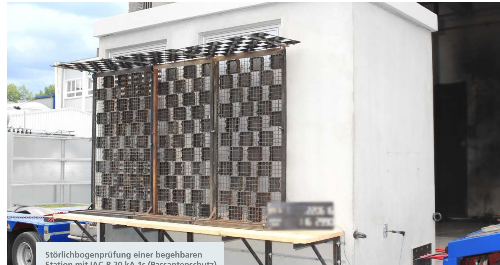
Fault arc test of a walk-in station with IAC-B 20 kA 1s (pedestrian protection)
